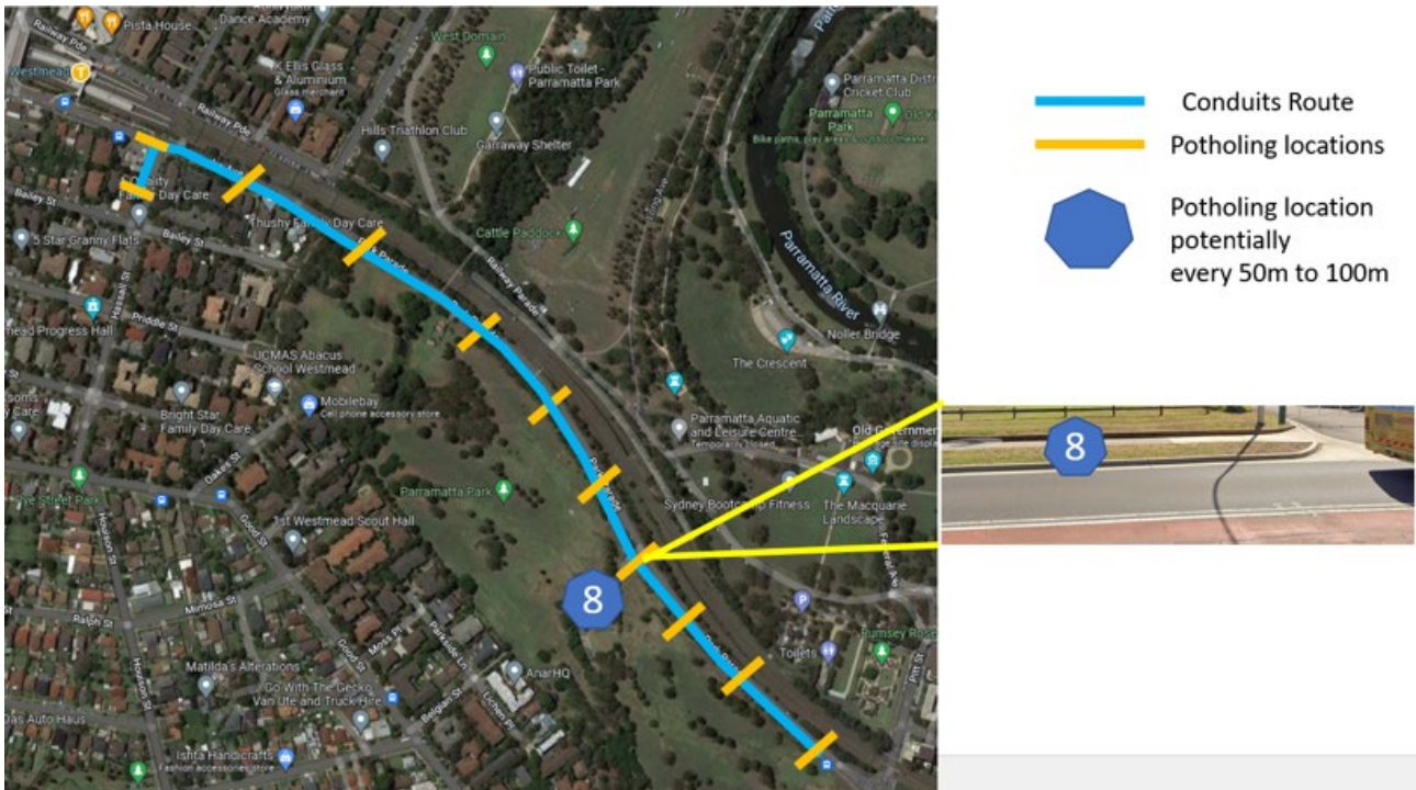
Figure 3-4: Indicative potholing locations along Park Parade/ Alexandra Avenue
