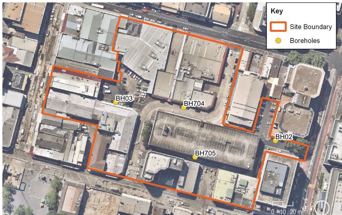
Figure 4.9 Location of geotechnical boreholes within and surrounding the site. The 'fill' depths are provided beside each location. (Source: Nearmap with GML overlay 2021)
