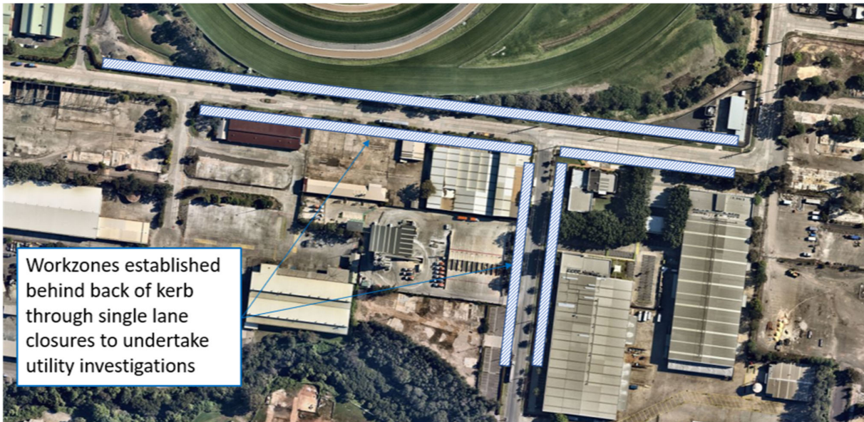
Figure 7-1: Unwin Street southern side work areas
