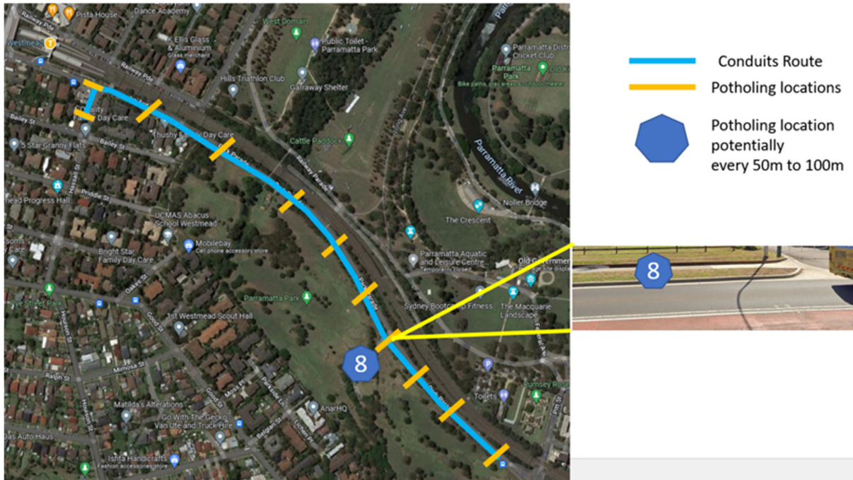
Figure 3-4: Indicative potholing locations along Park Parade/ Alexandra Avenue
