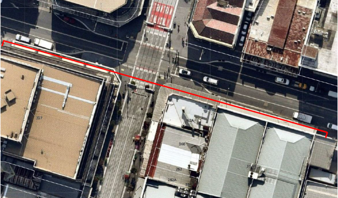
Figure 7-6: New power supply route
