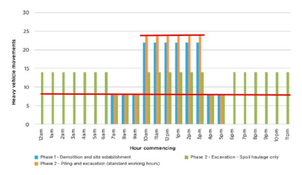
Figure 3-15: EIS hourly heavy vehicle movements (source: EIS Chapter 10 page 10-13)
