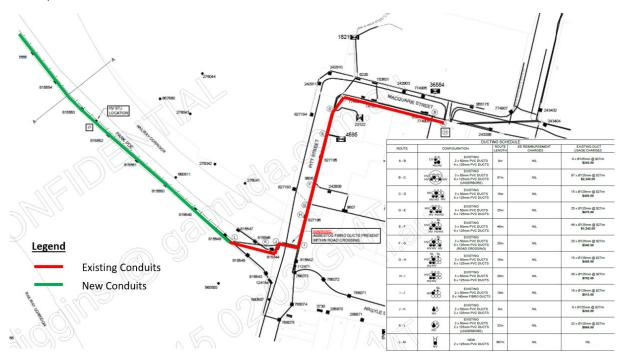
Figure 3-1: HV Power supply route - eastern end
