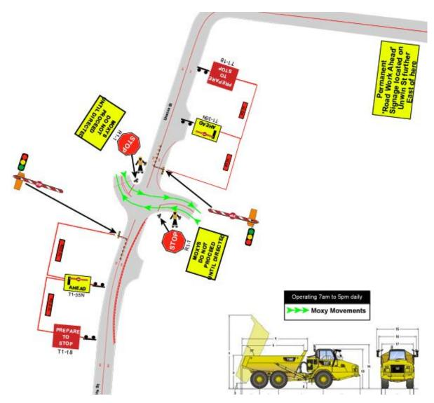
Figure 3-15: Haul road crossing on Unwin Street
