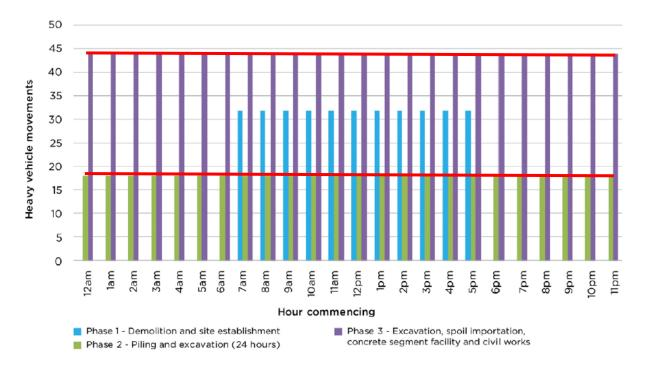
Figure 10-14: Hourly heavy vehicle movements at the Clyde stabling and maintenance facility construction site Note: Movement means a one way movement. A truck entering and then leaving a work site represents 2 movements.
