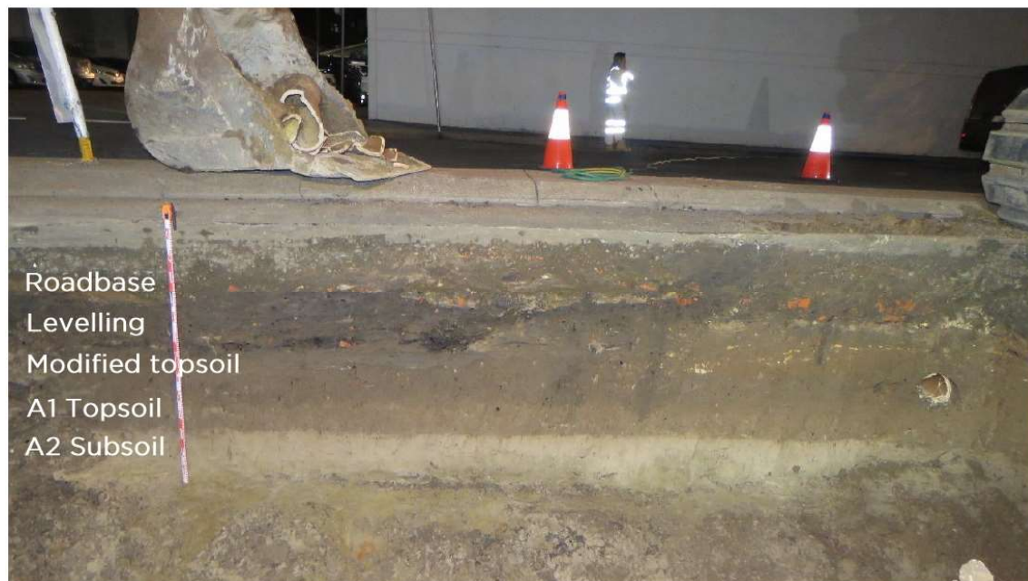
Figure 4.6 South-facing section in Test Trench 10 showing the intact soil profile below modern levelling fills. (Source: Casey & Lowe 2021)
