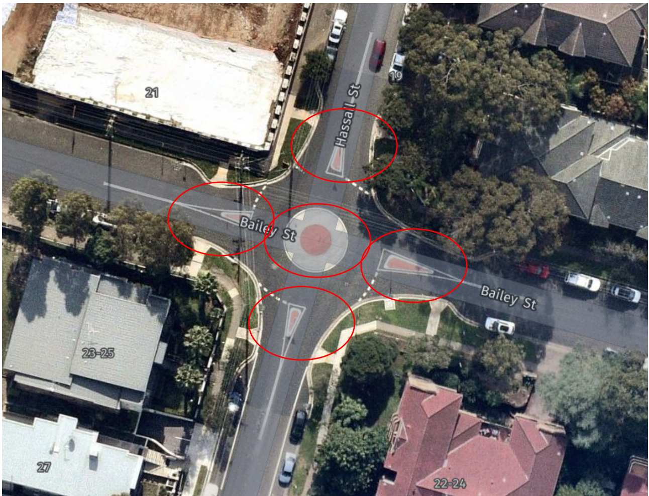
Figure 4-1: Roundabout and splitter islands to be removed
