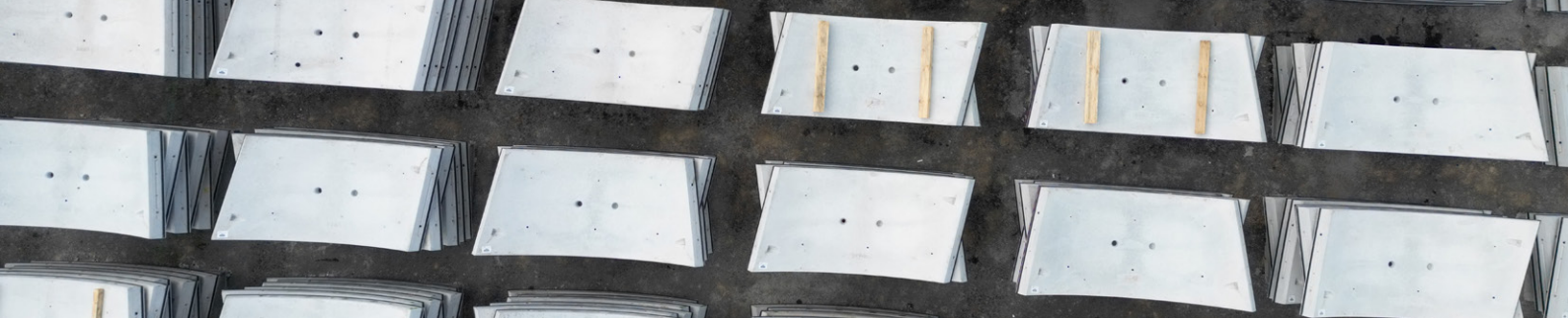
Precast concrete segments from the Project's Eastern Creek precast facility.
