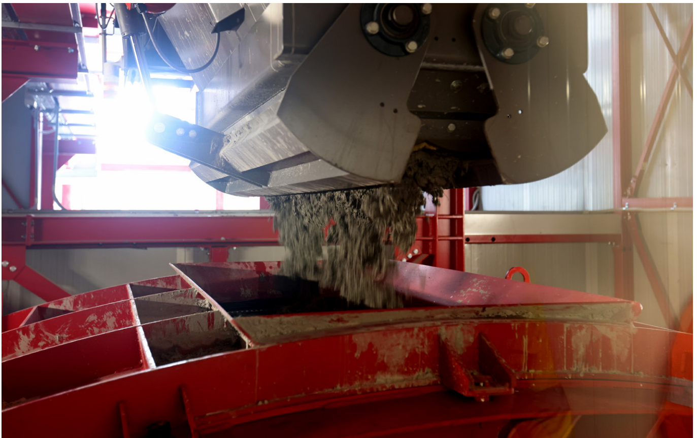
Segment production in progress at the Project's precast facility.
