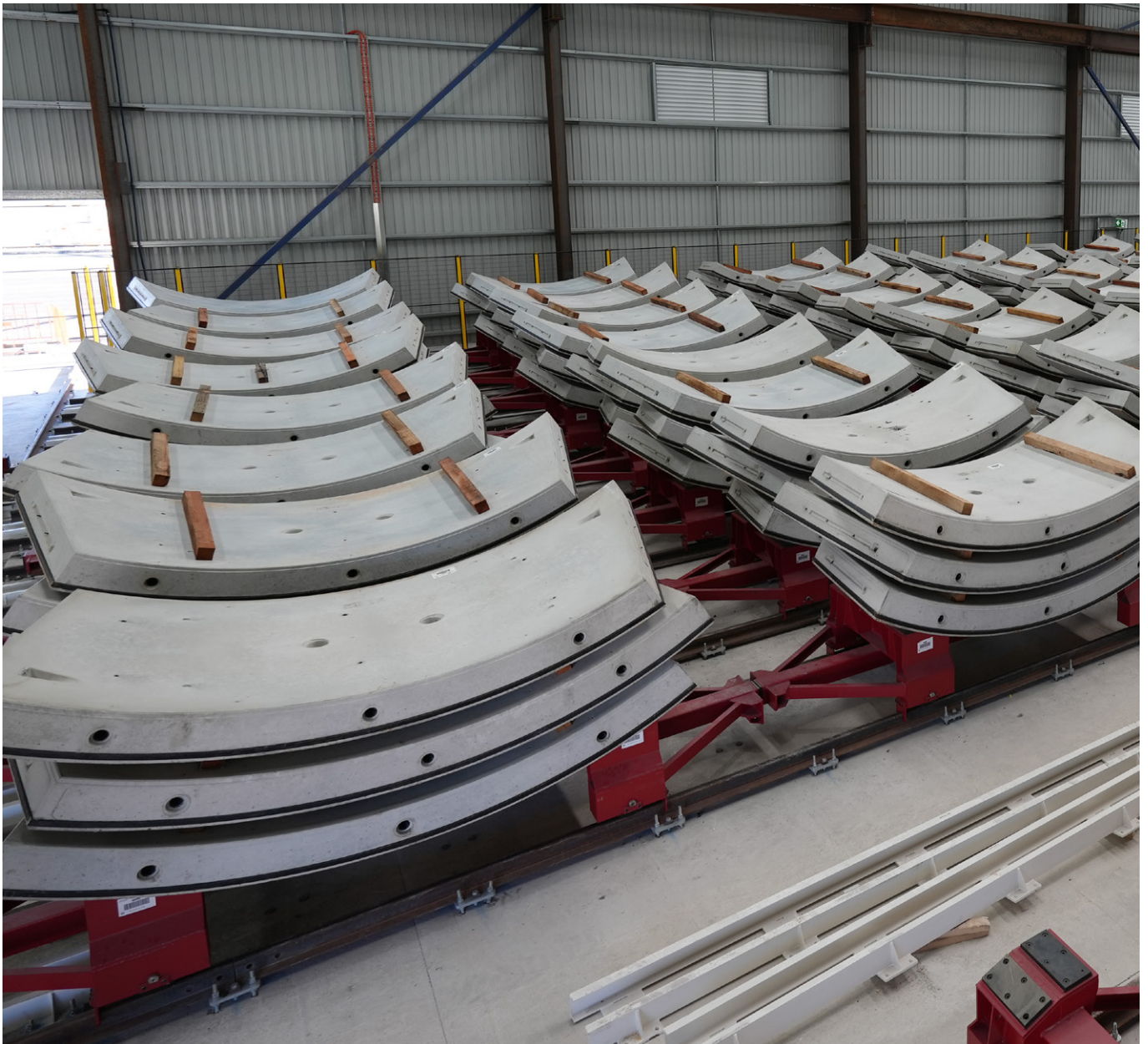
Precast concrete segments are transported from Eastern Creek to Clyde to line the Sydney Metro West twin metro tunnels.
