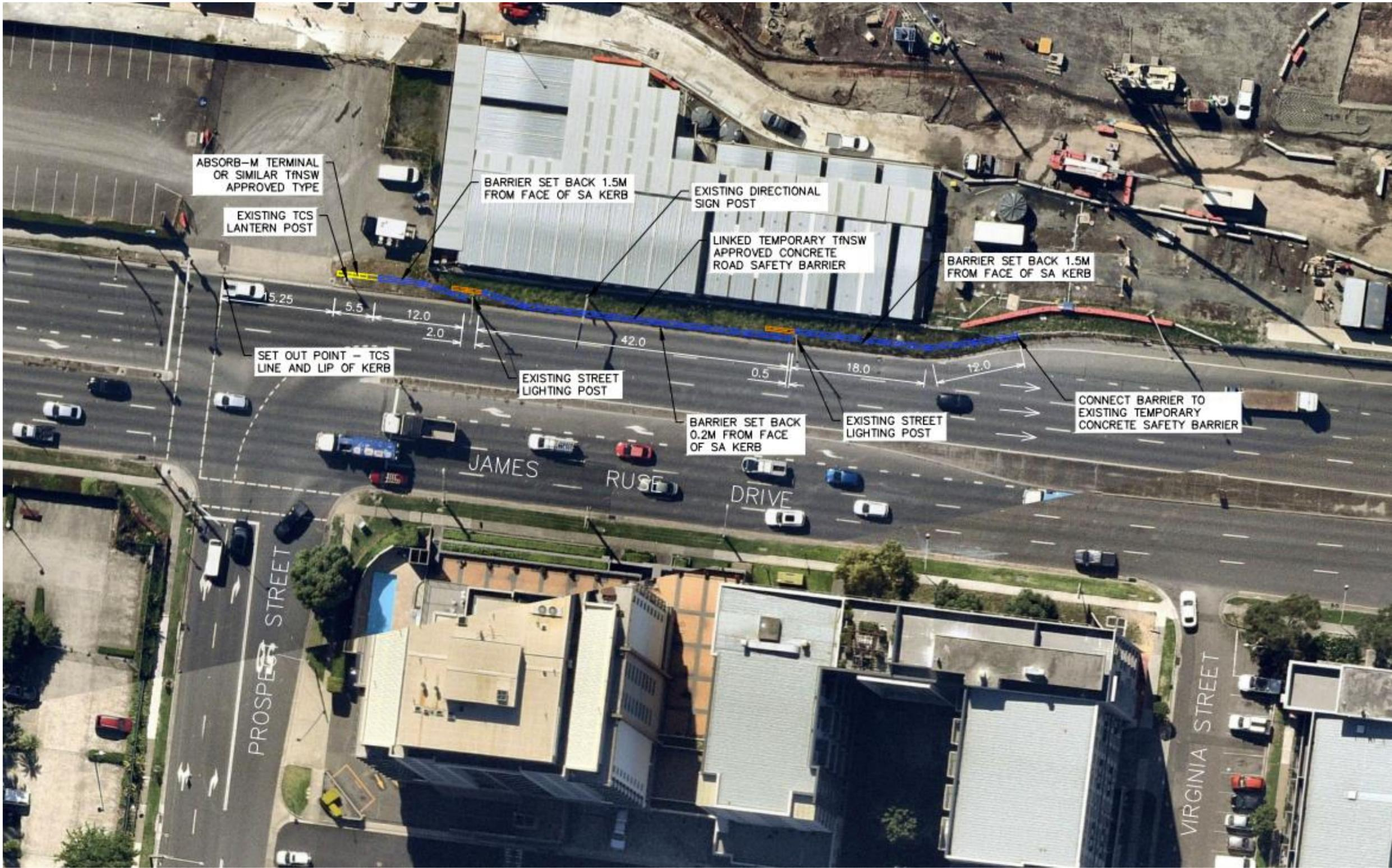
Figure 5 - Temporary safety barrier design
