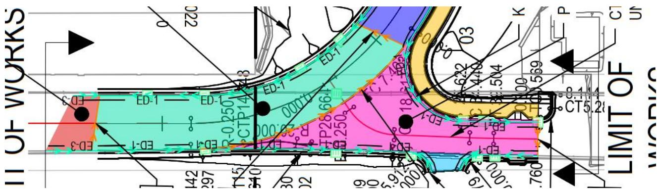
*Figure 5 - Indicative Diagram of Pavement Types*
