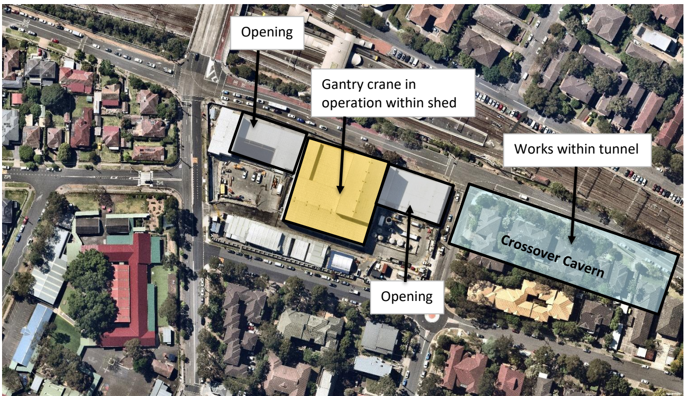
Figure 2 Location of Works – S2 (FRP Works – Steel Fixing and Falsework Operation)
