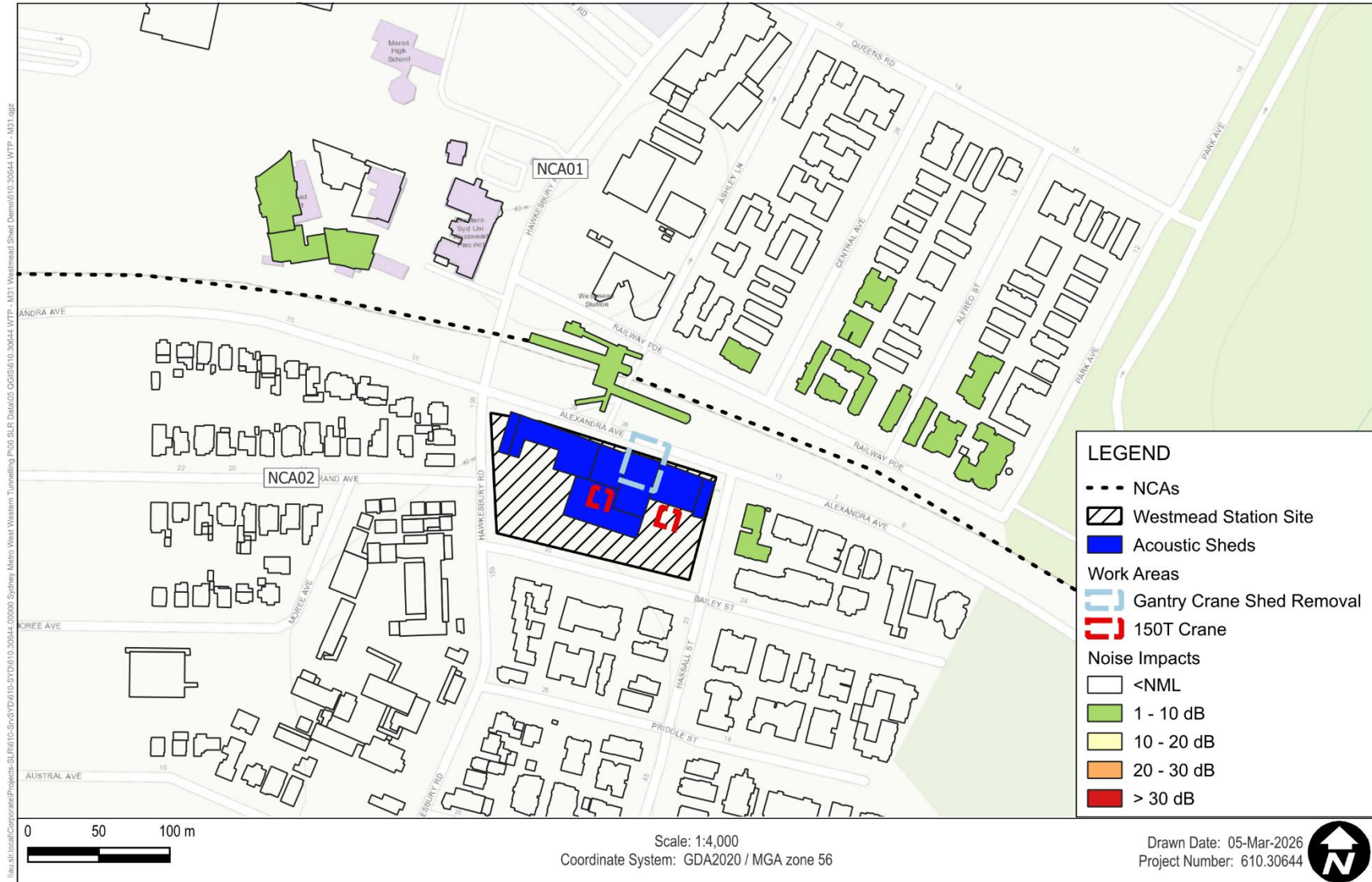
Figure A6 S6b – Shed Demolition (with 150 t Crane) – OOHW1
